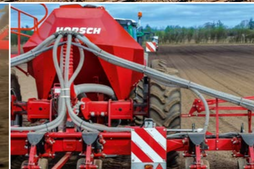
Seed wagon for 2 000 litre seed and 7 000 litre fertiliser for maximum efficiency
