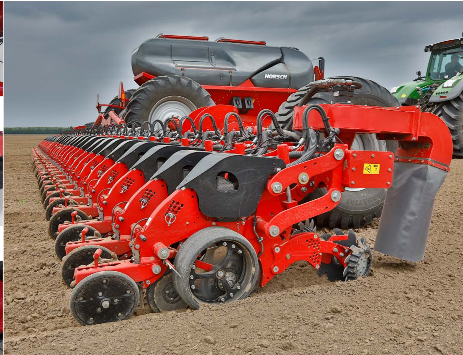
Maestro SW with liquid fertiliser unit to apply fertiliser on the seed row
