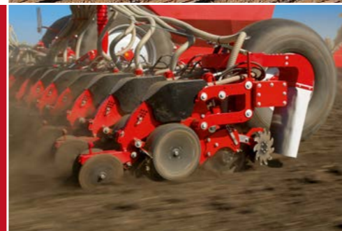
Extremely robust single grain seed units with precise grain singling and Seed on Demand system
