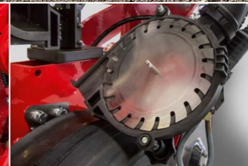
The new metering disc of the Maestro with open grooves
