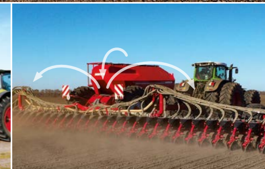
Transfer of the seed wagon weight to the seed bar for increased coulter pressure
