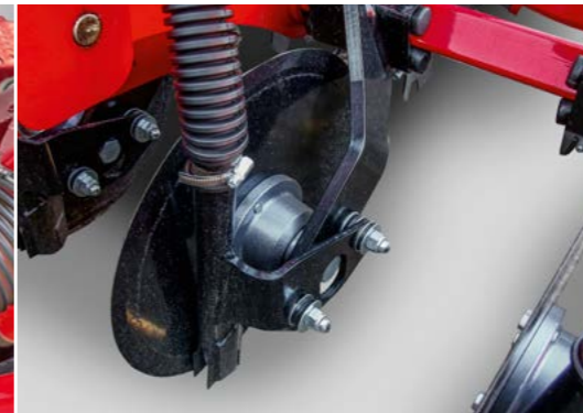
PPF fertiliser coulter Maintenance-free coulter with high coulter pressure
