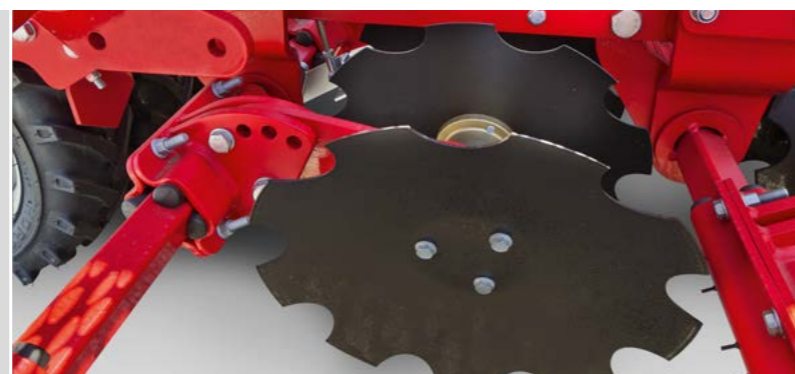
Disc adjustment as track eradicators (optional)
