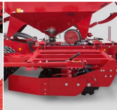
Adjustable side plates Ensures even levelling between passes
