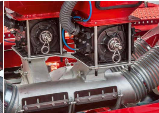
Double venturi for simultaneously applying fertiliser in one flow
