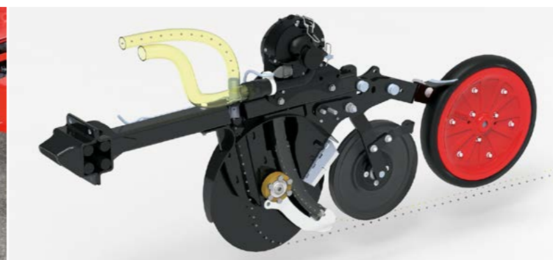
Placement of fertiliser and seed via two divided inlets – combines the advantages of single grain seed and contact fertilisation in rape and cereals
