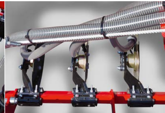
Variable depth adjustment Fertiliser placement between two seed rows, in the centre line of the tyre
