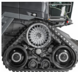
The TrakRide track tractor ensures exceptionally low ground pressure.
