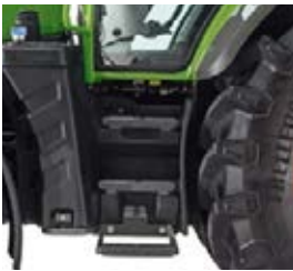
■ The steps are protected against dirt from the side. There are also wide steps and a well-placed handrail to get up and down safely. The door handle is easy to reach from the ground.
