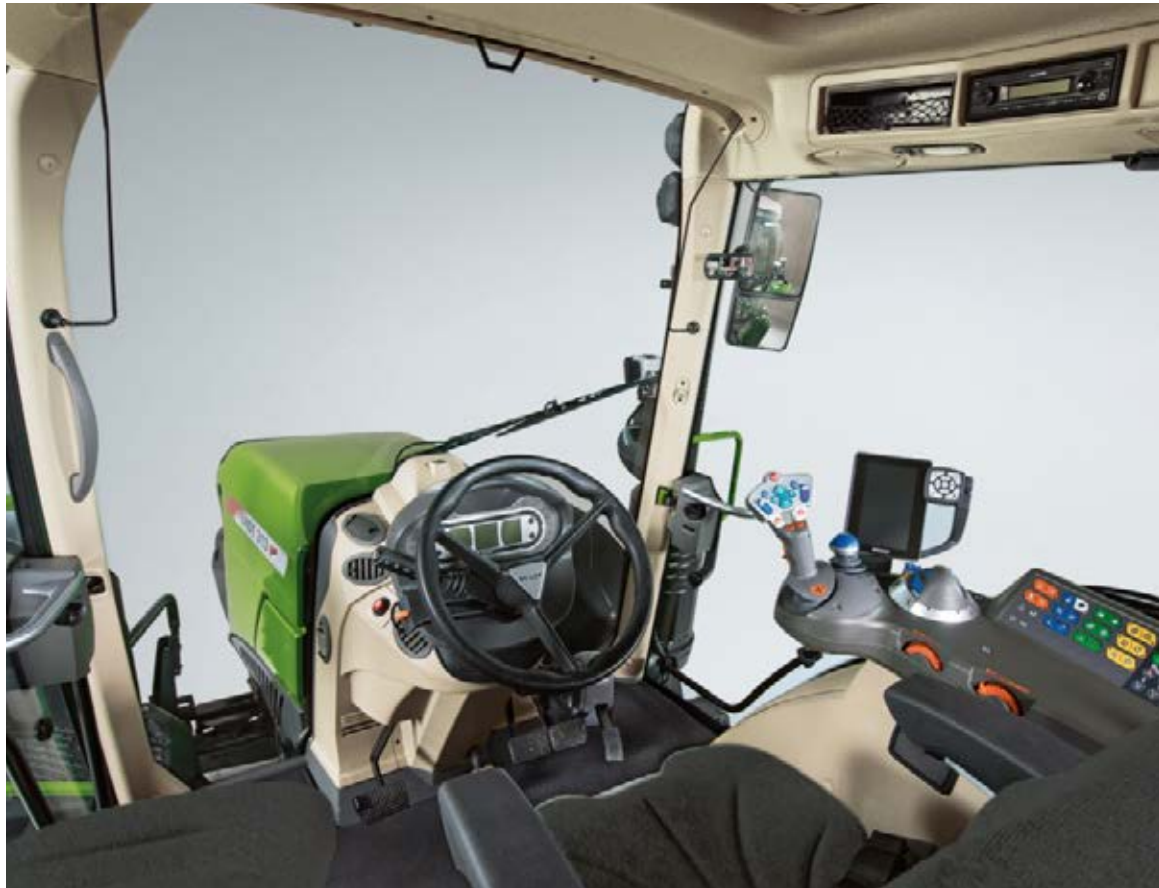
The clearly laid out and ergonomically designed VisioPlus cab offers the best overview, both to the operating elements and the field. The windscreen comes either as a continuous panoramic window or as a hinged pane. You can choose a second door in place of the right side panel.
