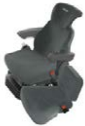
■ The comfort seat features air suspension and easy armrest adjustment.
