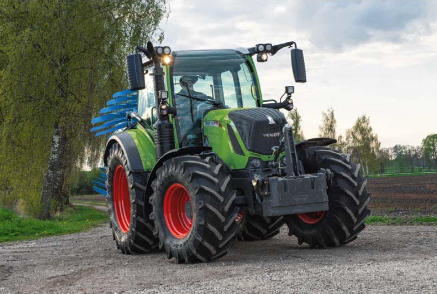
Engine characteristics – Fendt 300 Vario The high 596 Nm torque and 143 hp maximum power at 1,750 rpm ensure full engine power and agility.
