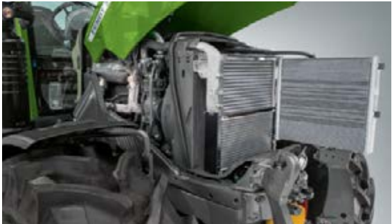
Less to do, leave work earlier: The compact radiator package is very accessible and can be cleaned easily and quickly because of the generous clearance between the coolers and the flat radiator bottom.
