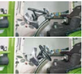
Steering wheel and cockpit perfectly adjustable by foot pedal: For the best sitting position, the steering wheel and cockpit must be at the right height and tilt angle.
