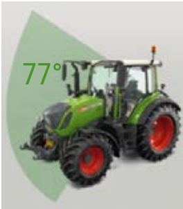
Panoramic windscreen with 77° vision for a full view upwards and over the wheel arches.
