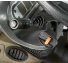
Particularly practical: The indicator reset has 3 trigger settings: steering angle, time and speed.
