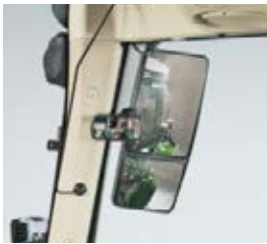
■ The wide-angle mirror is integrated into the main mirror as a second mirror and considerably increases your field of vision.
