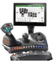
Power+ Setting 1 - Crossgate lever - One rocker pair (linear module) to control the hydraulic valves
