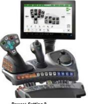
Power+ Setting 2 - 3L joystick - One rocker pair (linear module) to control the hydraulic valves
