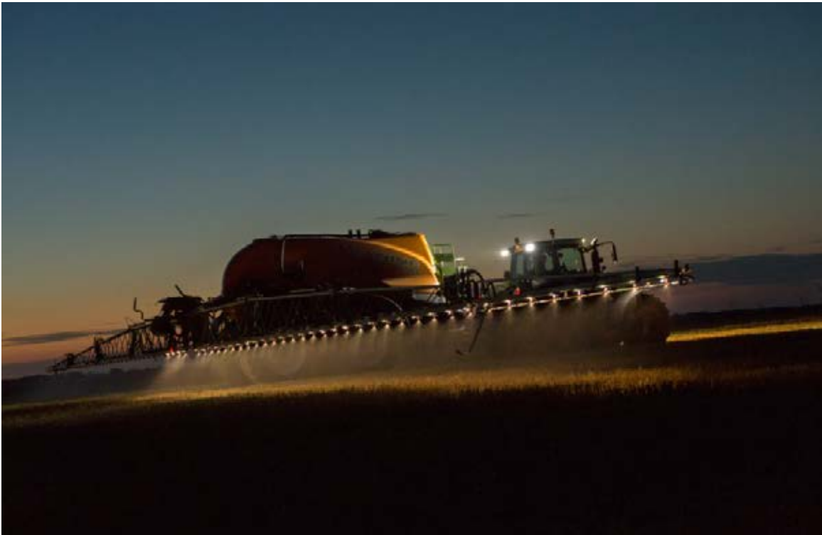
State-of-the-art lighting: The 360° lighting design concept on the Fendt 800 Vario has been perfected and is state-of-the-art. The dipped and main beams have the latest Bi-LED lamps with headlamp levelling. The work lights and corner lights are also fitted with LED lamps. This permits precise control of the illumination and provides exceptional visibility to the implements and the wheel arches, even in the dark. The LED lights are especially low in power consumption, have a very long life and deliver a total luminous flux of up to 49,900 lumen.
