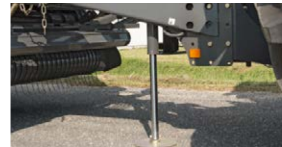
The optional hydraulic parking jack makes light work of attaching and detaching the tractor.
