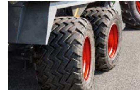
Steering tandem axle for high manoeuvrability.
