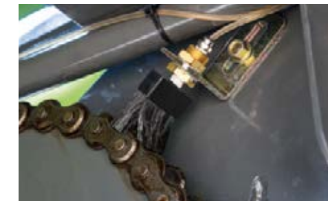
Automatic chain lubrication of all the most important drive chains is new. The lubrication intervals can be conveniently set via the terminal.
