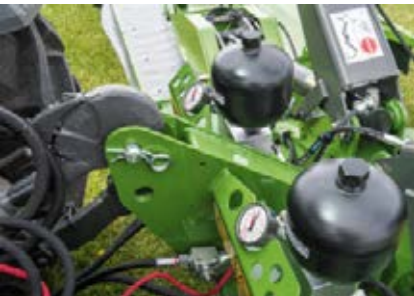
Always keep an overview of the perfect TurboLift system contact pressure using the field pressure gauge, and adjust it from the comfort of your cab.
