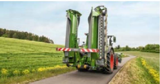
When folded, the mower combination remains below 4 m in height, and can be easily driven thanks to the low centre of gravity.
