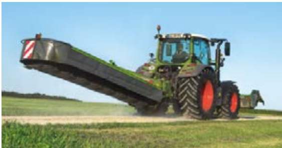
The mower swings through 90° to the rear from the cab in the transport position.
