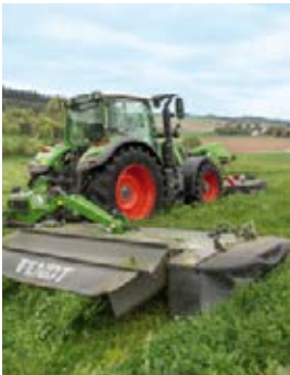
Using the pivot, the mower units can be adjusted to follow the ground perfectly.
